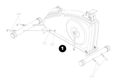
**1.** Attach foot tubes (4) to the frame by using the carriage bolts (44), flat washers (50) and cap nuts (45) provided. Make sure the foot tube with wheels is assembled onto the front of the unit.
